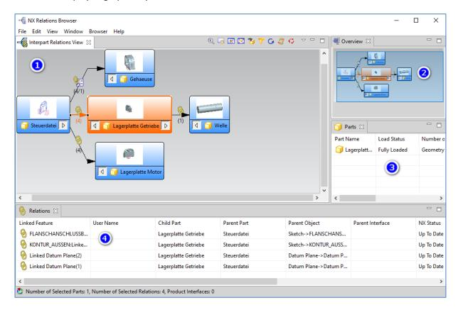
(1) The parts and links are displayed graphically in the "Interpart Relations View" window. The content to be displayed is defined in the "View" pull-down menu:
